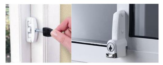
Window pins and bolts work much like deadbolts on doors. A lock mechanism with a sliding bolt or pin is fastened to the window sash or frame so that the bolt slides into a receiver (like the deadbolt would slide into a strike plate). You can also find a design where the bolt slides into a hole drilled in the window sash or frame. The lock and the receiver are usually aligned for easy operation.
